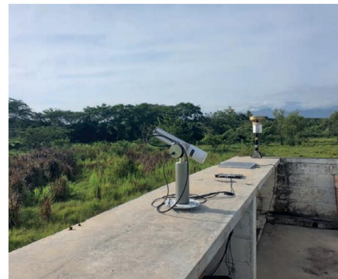
Image 1 - View of the sunphotometer while performing measurements
